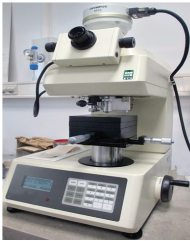
Fig. 2: Surface microhardness measured using a Vickers diamond indenter
