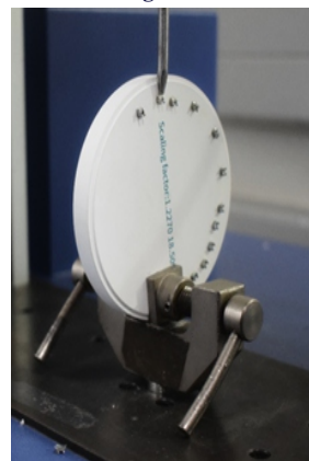
Fig:8- ceramic block with brackets bonded placed in Instron Universal testing Machine to test shear bond strength
